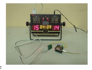
ESP32 has been updated with the correct IP address for the Raspberry Pi, the ESP32 can then be powered by any micro USB cable supplying five volts. A picture of the connections for scoring integration can be seen above.
